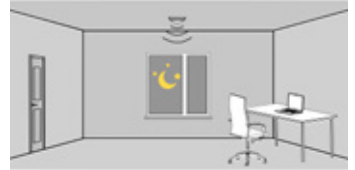
No presence detected, lights off
