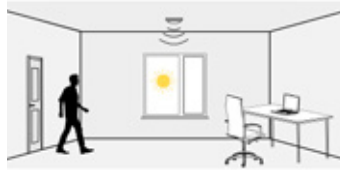
Presence detected, sufficient daylight, lights off
