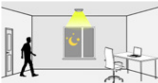
1. The light switches on at 100% when there is movement detected.
