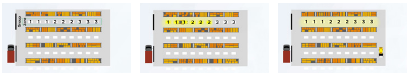
1. Luminaires can be grouped together or further divided into zones
