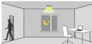
2. The light dims to stand-by level after the hold-time.
